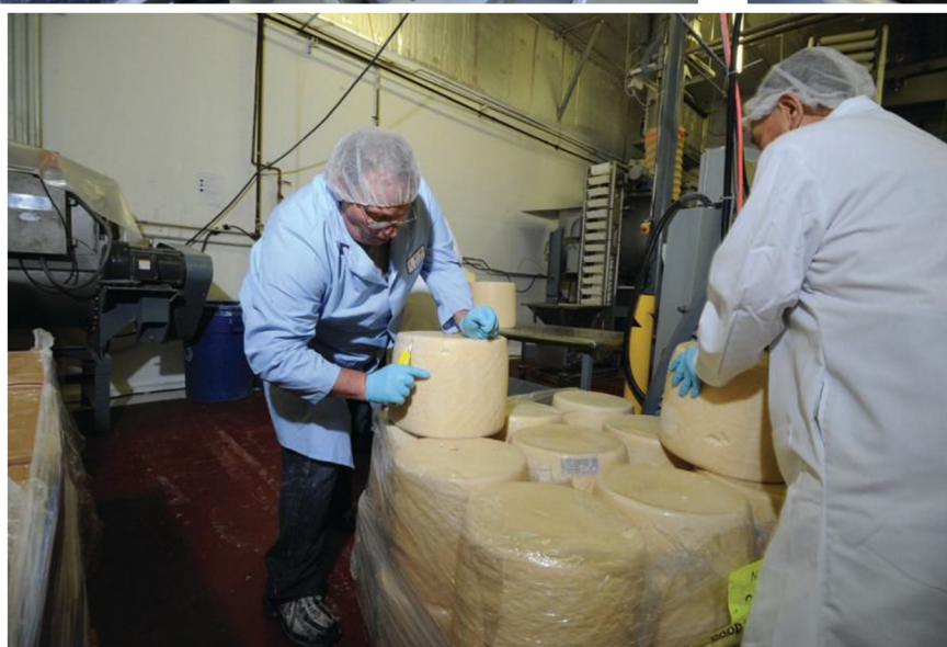
■ Top left: After being chopped, a conveyor lift moves product into the vibratory conveyor, which travels into the packaging area. Left: Cheese comes in from various domestic and imported suppliers in wheel forms (in a multitude of sizes), which are sliced in halves and then sent through a bowl chopper. Above: While in the chopper, which holds 500 pounds of mix, operators add an anti-caking blend to protect the product.
