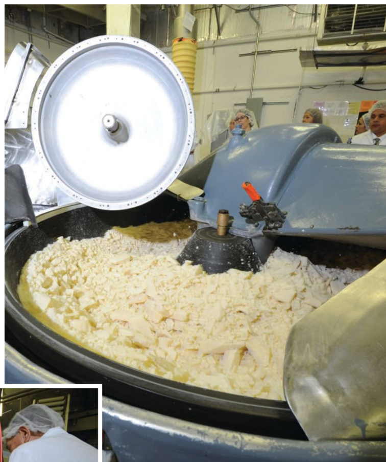
■ Top left: After being chopped, a conveyor lift moves product into the vibratory conveyor, which travels into the packaging area. Left: Cheese comes in from various domestic and imported suppliers in wheel forms (in a multitude of sizes), which are sliced in halves and then sent through a bowl chopper. Above: While in the chopper, which holds 500 pounds of mix, operators add an anti-caking blend to protect the product.
